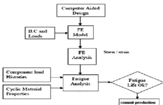
**Figure 6.** The finite element based fatigue analysis cycle
