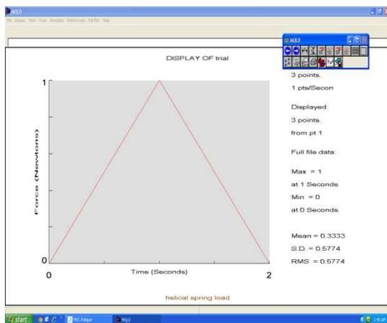
**Figure 7.** Fatigue load curve (Nastran)
