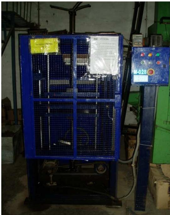
**Figure 4.** Spring fatigue testing machine
