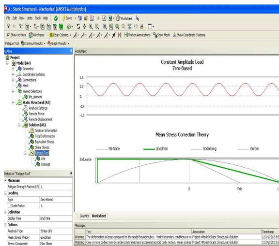
**Figure 9.** Fatigue load curve (Ansys)
