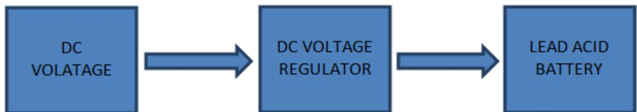
**BLOCK DIAGRAM OF CHARGER FOR LEAD ACID BATTERY****Observations:**
