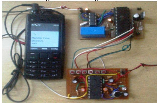
Fig5. Design of Main Circuit Diagram of Monitoring Of Flow Control Using Mobile
