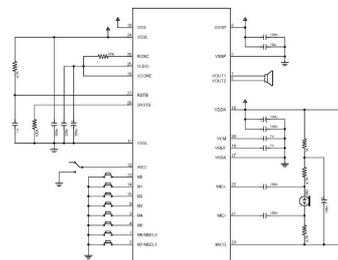
Fig3.IC Apr33a3 Audio Recording and Playback Circuit
