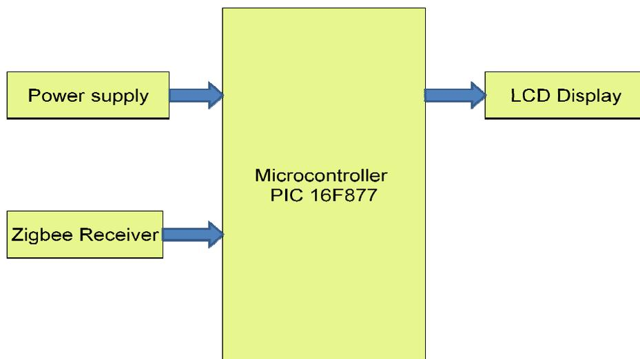
Figure 2: Block diagram of Receiver
