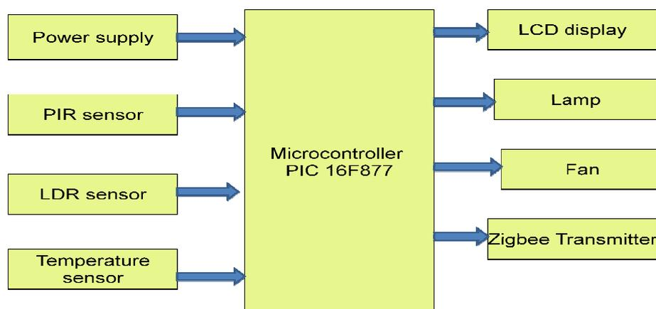
**Figure 1: Block diagram of Transmitter**
