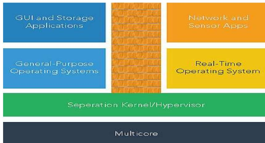
**Figure 2:** Embedded virtualization example for real-time data sensor sampling and GUI management and reporting.
