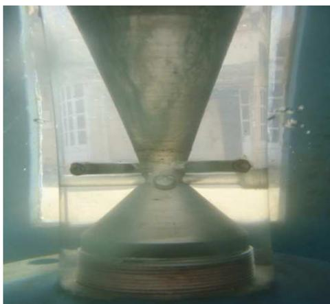
**Fig. 2:** Venturi Scrubber machined of acrylic material
