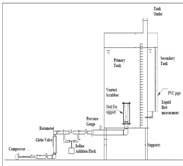
**Fig. 5:** Experimental setup prototype (Configuration I)
