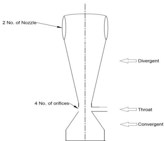
**Fig. 1:** Schematic of venturi scrubber
