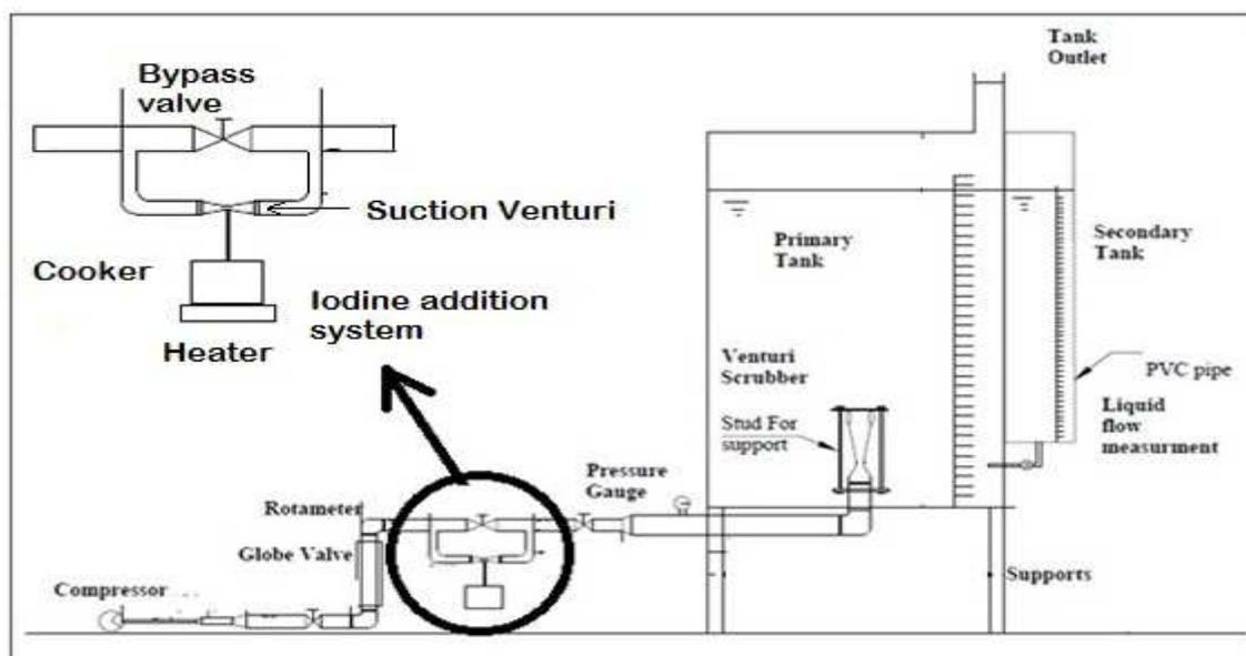
**Fig. 4:** Experimental facility to carry out the experiments of iodine removal efficiency
