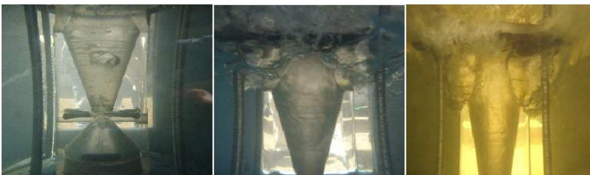
**Fig. 3:** Removal phenomenon in Venturi Scrubber due to atomization of scrubbing liquid
