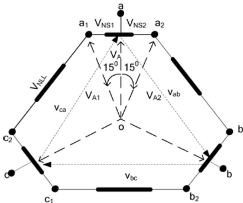
Fig 3. Phasor and Winding diagram of proposed 24 pulse Auto transformer
