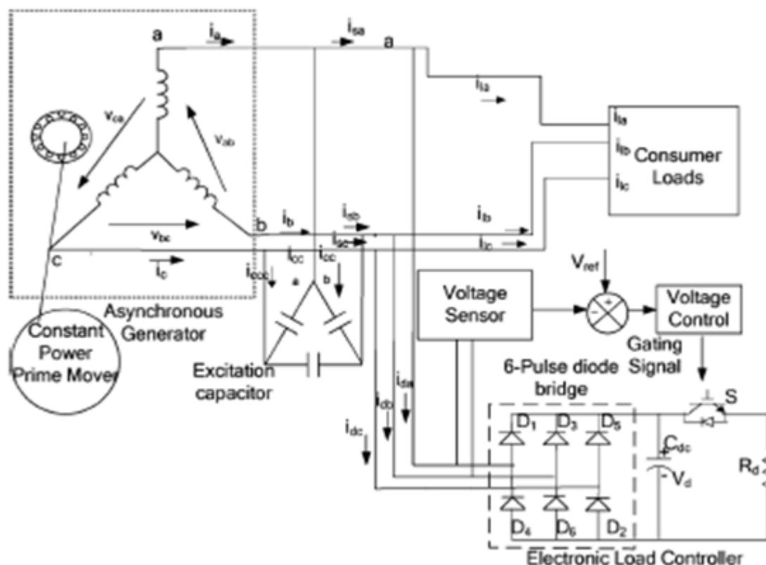
**Fig 1. IAG system configuration and control strategy**
