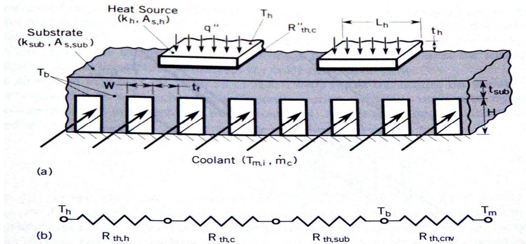
Fig 2: Thermal Resistance network for Heat sink analysis.
