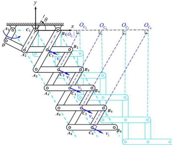
Foldable stair is easily deployed for use and folded for storage. It consists of a number of identical deployable scissor-like elements which form the staircases when expanded. In addition to use, the folded stair can be used for up & down motion of weapons.
